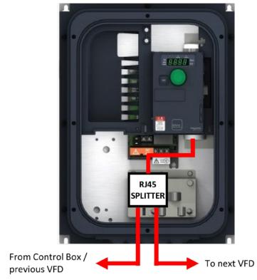
\*Connect Cat5 Cable and splitter to port inside of VFD enclosure
